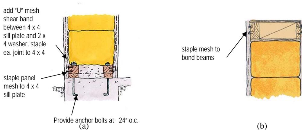
Figure 4. Recommended anchorage details (a) at the base of the wall and (b) at the top of the wall.
