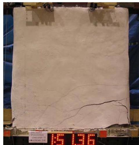
(f) Flexural cracks in Wall F (2.5% drift)
