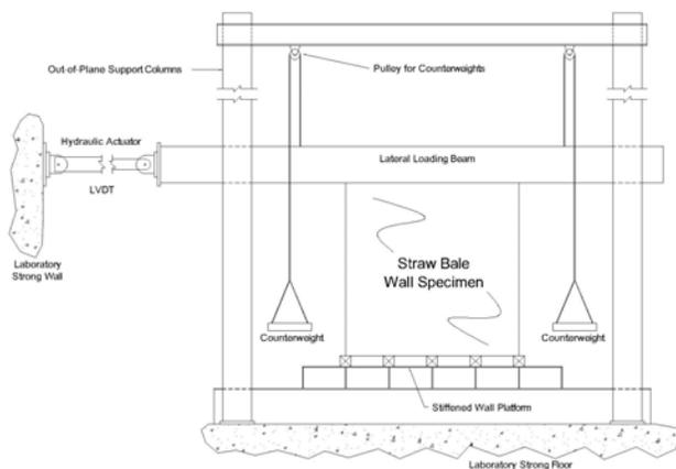
Figure 7. Test setup
