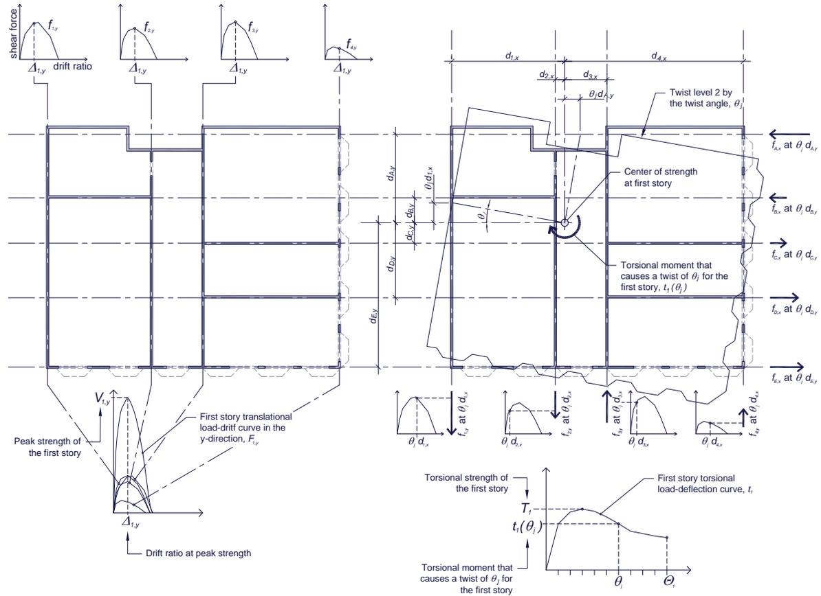
**Figure 3.3.** Left, illustration of procedure to compute translational backbone curve. Right, illustration of procedure to compute torsional backbone curve.
