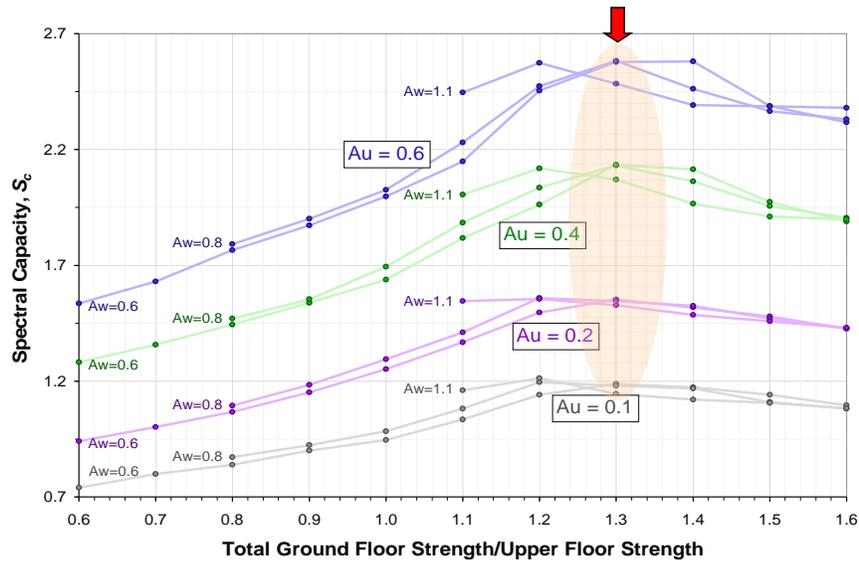
**Figure 2.5.** A plot showing the trend of Spectral Capacity with increasing ground-story retrofit (quantified by weak-story ratio,  $A_w$ ) for various families of upper structure strength ratio  $A_u$ . Peak spectral capacity for all families occurs around  $A_w = 1.3$ .
