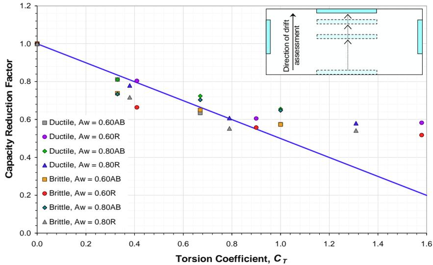
**Figure 2.6.** Plot of Torsion Coefficient,  $C_T$  versus reduction factor (relative to the base case with no torsion). Analytical models with various amounts of torsional imbalance were subjected to bi-directional input for the incremental dynamic analysis (IDA). The straight line conservatively applies a capacity reduction at very high level of torsional imbalance.
