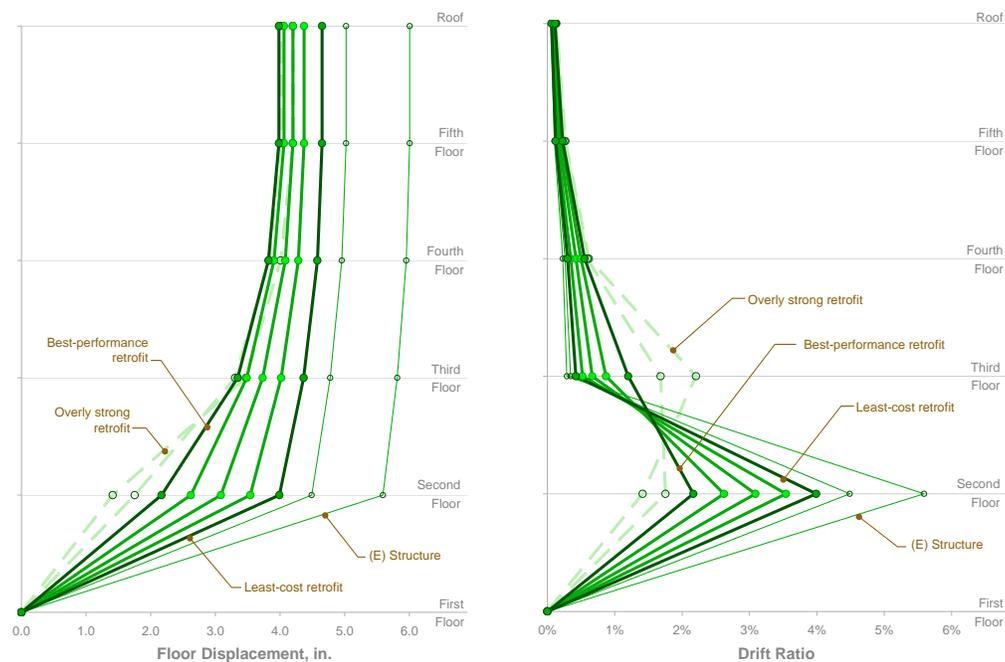
**Figure 2.1.** Displacements (left) and interstory drift ratios (right) are plotted for an archetype building, showing the unretrofitted condition and that of several retrofit options. The retrofits are new ductile elements of various strengths, located only in the ground story. The Relative Strength Method recognizes that there is a limit of capacity set by the upper structure.
