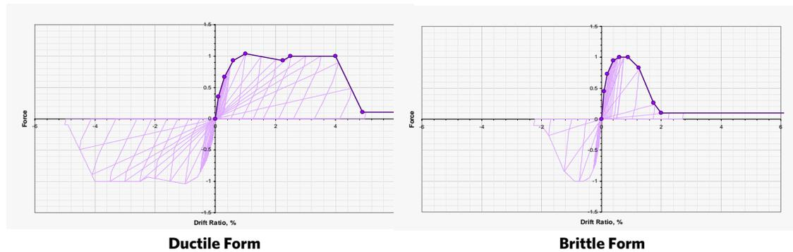
**Figure 2.4.** The backbone curves and hysteretic loops used in the IDA for the ductile form (left) and brittle form (right) of the structures.
