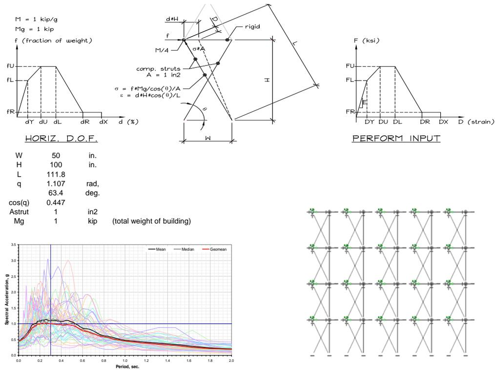
**Figure 2.3.** Illustration of models used in the incremental dynamic analysis. The vertical elements in the five structures in the lower right are for dead load to capture P-delta effects. These models were built in CSI Perform. The earthquake inputs were the FEMA P-695 far field record set shown in the lower left.
