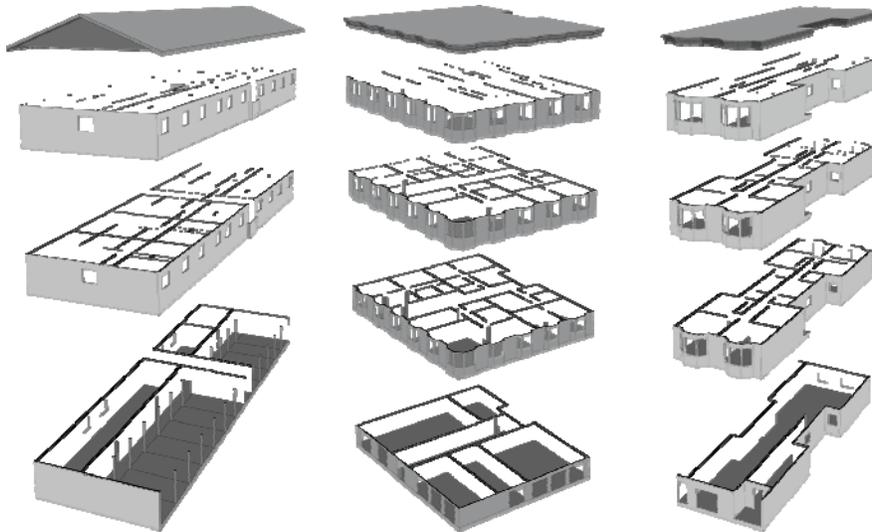
**Figure 1.2.** Diagrams of three archetype weak-story structures show the upper structure with numerous interconnected walls. Note lack of walls in the ground story, due to parking and commercial uses.
