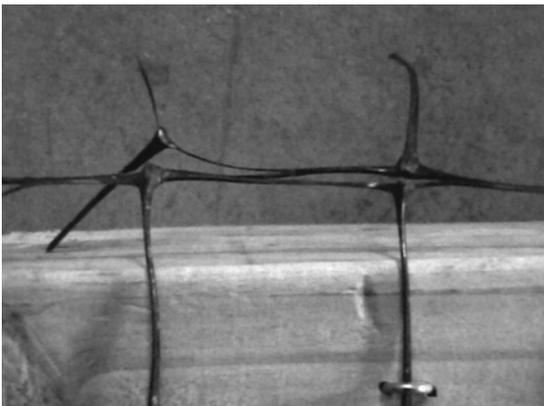
The lower strength polypropylene and hemp meshes were adequately anchored by the staples used in Configurations F, G, H, and I. A splitting failure of the polypropylene strand is shown in Figure 8. Unraveling of the hemp twine is shown in Figure 9.
