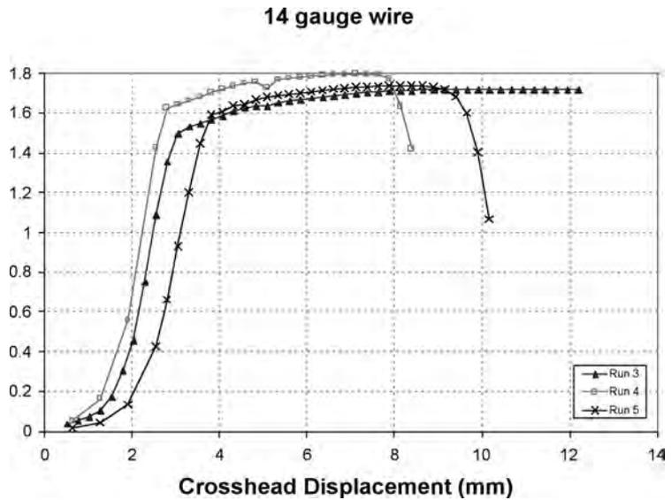
The measured diameters and corresponding areas of Table 1b correspond well to the American Steel & Wire (AS&W) reference standards for #14 and #16 gauge wire. The AS&W values for diameter are 0.0800 and 0.0625 in. (2.03 and 1.59 mm) and for area are 0.00503 and 0.00307 in<sup>2</sup> (3.24 and 1.98 mm<sup>2</sup>) for the #14 and #16 gauge wire sizes, respectively.
