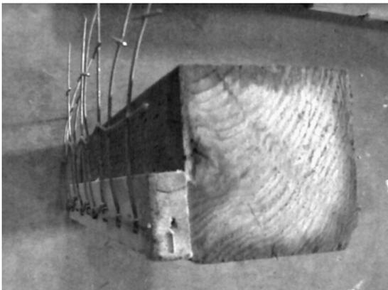
**FIGURE 4.** (a) detail showing alternating staples and sequence of individual wire tests; (b) test setup.
