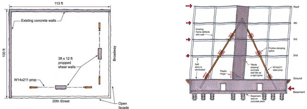
Figure 2. Plan and frame elevation of the propped shear wall retrofit.
