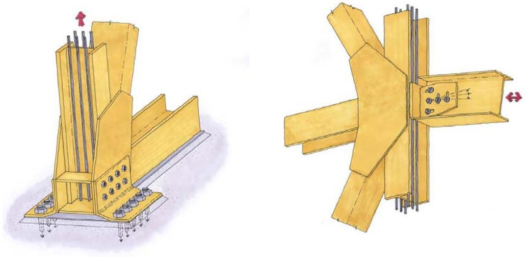
Figure 8. Post tensioned braced frame details. The base of the frame on the right is illustrated in the lifted position with the angles yielding in double curvature. The collector to frame connection on the right shows a pin configuration made up of slotted holes to accommodate the rocking.
