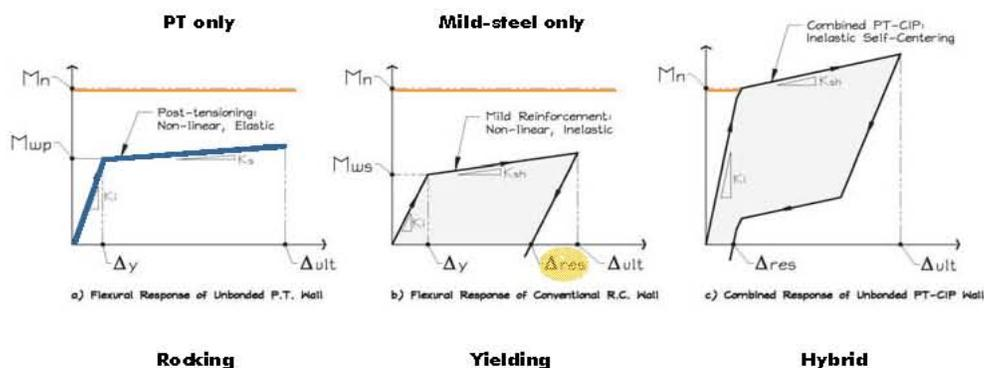
Figure 13. A simple model to describe the hysteretic behavior of PT wall systems as the sum of non-linear elastic rocking plus elastic plastic responses.
