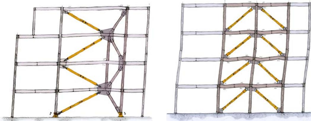
Figure 6: Trussed mast frame (left) with half the BRBs of a conventional chevron frame (right).
