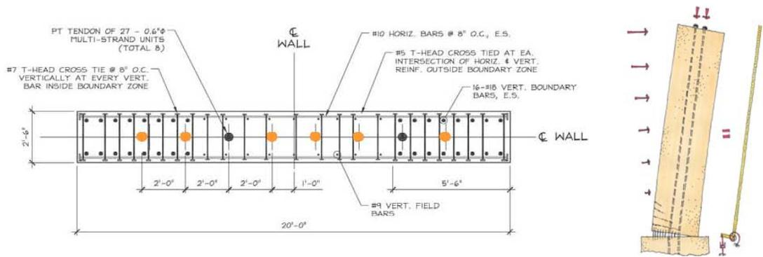
Figure 12. Post tensioned concrete flexural wall section and elevation.
