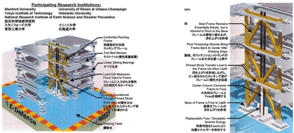
Figure 10. Illustration of post tensioned rocking frames tested at E-Defense in Japan.
